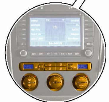
Climatronic control unit J255, in middle of dash panel
